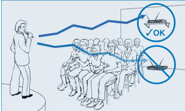
proper and improper antenna and receiver placement
